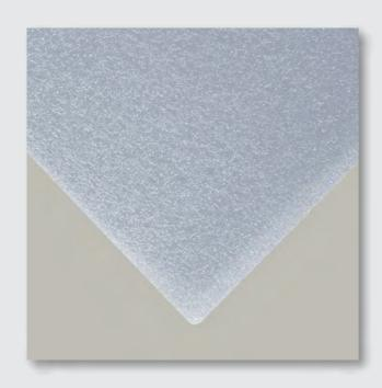
**THICKNESS** 2 mm **ROLLS** H 1200 mm X L 25 mtl **DIMENSIONAL** ± 10% **TOLERANCE THERMAL**  $\lambda = 0.045 \text{ W/mK}$ **CONDUCTIVITY** REDUCTION OF 19,0 dB **IMPACT NOISE COMPRESSIVE** 4 KPa (10%); **STRENGTH** 17,5 KPa (25%); 62 KPa (50%) RESISTANCE Thickness d'aria TO VAPOR equivalente  $S_d > 4 \text{ m}$ **COMPRESSION**
