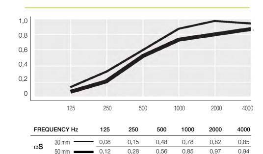
Determination of sound absorption coefficient according to DIN 52212 in large reverberation room
