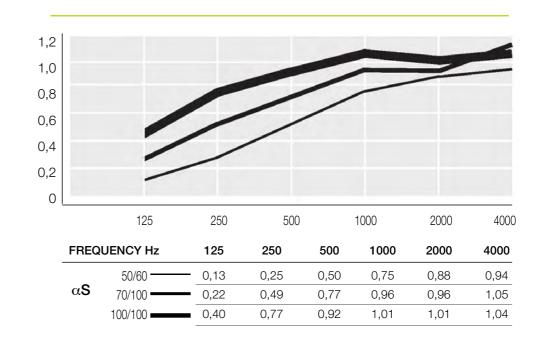
Determination of sound absorption coefficient according to DIN 52212 in large reverberation room
