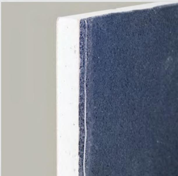
LA LASTRA IN CARTONGESSO, ACCOPPIATA SU UN LATO CON UN PANNELLO FONOSOLANTE IN POLIETILENE CON INTERPOSTA LAMINA DI PIOMBO
