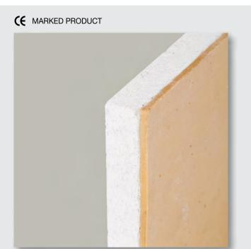
SPECIAL GYPSUM FIBER BOARD WITH A 12,5 MM THICKNESS AND WEIGHT OF 15 KG/M<sup>2</sup> COMBINED WITH AN EPDM TECSOUND® HIGH MASS LAYER OF 5 KG/M<sup>2</sup>
